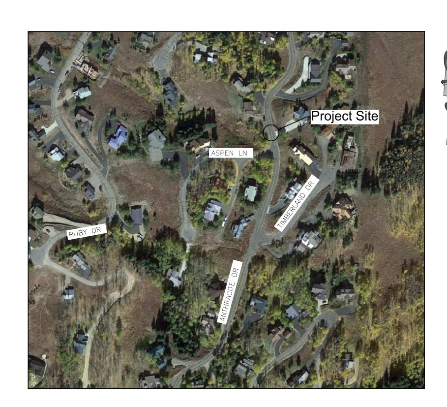
This project includes the remediation of a roadway slump along Anthracite Drive (Lower Slump). Remediation includes improving drainage, installing a culvert and underdrains, installing a culvert, and removal and replacement of existing fill materials with a modified reinforced soil slope (RSS) embankment. The work also includes hot mix asphalt paving and a concrete valley pan.
